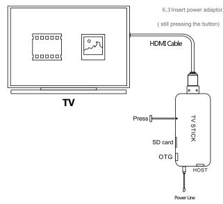
6.4 You can stop pressing the reset button until you see the android robot. And use
